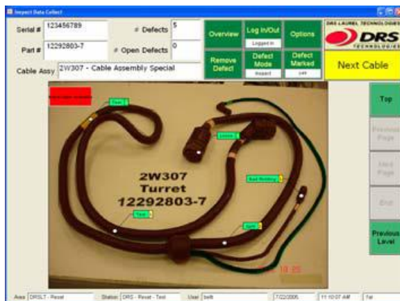
Green flags indicate finished repairs
